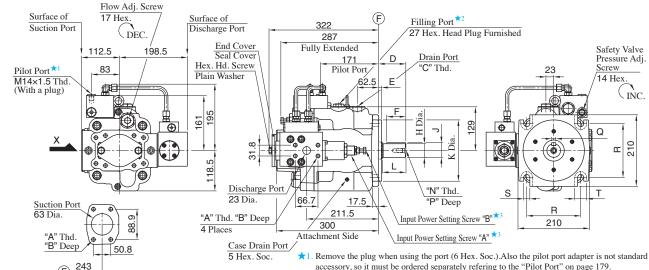
accessory, so it must be ordered separately referring to the "Pilot Port" on page 179. ★2. Install the pump so that the "Filling Port" is at the top.
