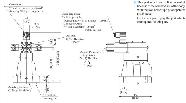
Note: For valve mounting surface dimensions, see the dimensional drawings of sub-plates (p.213) in common use.
