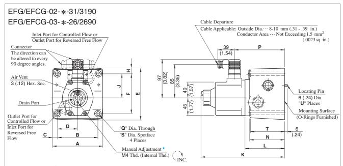
★ Manual adjustment can be done by screwing for example an M4×20 L screw in the M4 thread or pushing in a rod etc. there.
