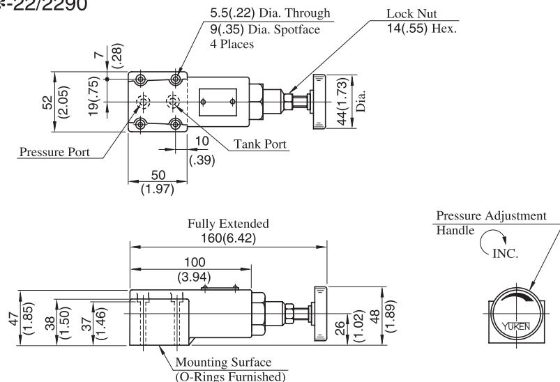
Note: For dimensions of the valve mounting surface, see the dimensional drawing (page 204) of the sub-plate used together.
